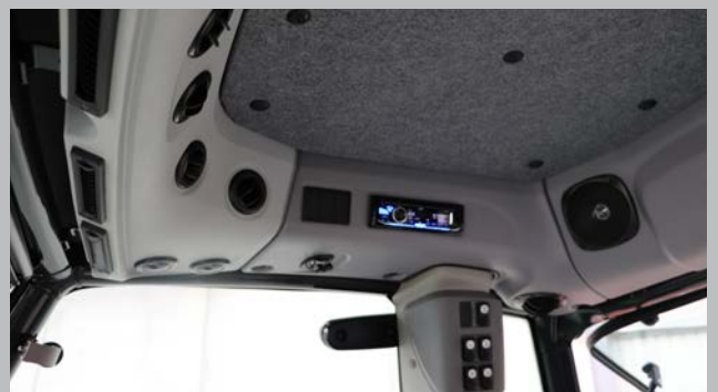
Air vents located throughout cabin.
